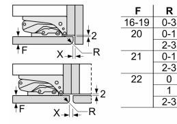
The gap dimensions recommended in the table must be adhered to in order to ensure that appliance doors do not collide with anything when they are opened, and to avoid causing damage to kitchen units.
