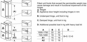
B: Undamped hinge, unit front in kg C: Damped hinge, unit front in kg D: Additional possible load in kg with heavy load kit
