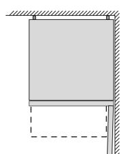
If the appliance is fitted directly to the wall, all of the drawers can be pulled out fully.
