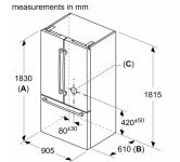
A: Front is adjustable from 1830 to 1847, with front levelling feet fully extended
