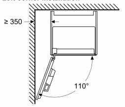
If using the 92° hinge limiter, the min. distance to the wall is only 100 mm  $\,$
