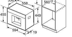
Bean and water containers are removed from the front. Recommended installation height 95-145 cm. measurements in mm
