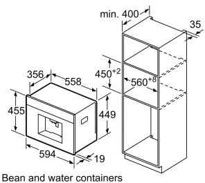
are removed from the front. Recommended installation height 95-145 cm. measurements in mm
