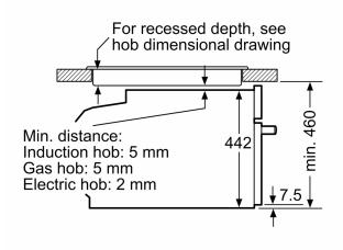
measurements in mm
