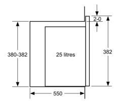
measurements in mm
