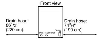
The electric connection socket and the water inlet are located on the front of the appliance, the outlet on the rear.
