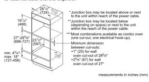
Flush installation Steam convection oven over single oven\*\*
