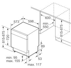
measurements in mm
