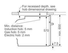
measurements in mm
