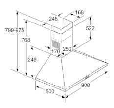
measurements in mm
