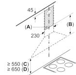
A: Socket B: Exhaust air: ≥ 280; circulated air: ≥ 490 C: electric D: Gas, from upper edge of pan support
