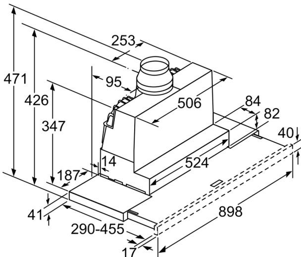
Depth of the filter drawer can be adjusted by up to 29 mm
