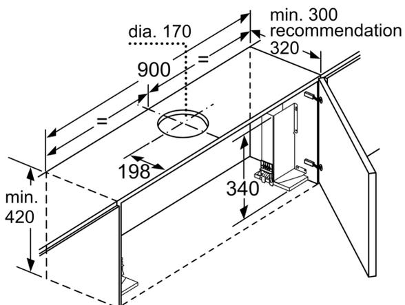
When installing the 90 cm telescopic hood in a 90 cm wide wall-hanging cupboard, a mounting kit is required. The two mounting brackets are screwed onto the left and right of the kitchen unit. Installation in accordance with template.
