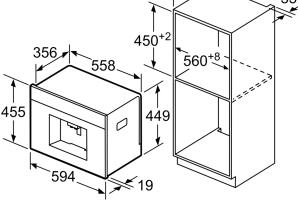
Bean and water containers are removed from the front. Recommended installation height 95-145 cm. measurements in mm
