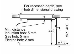
measurements in mm
