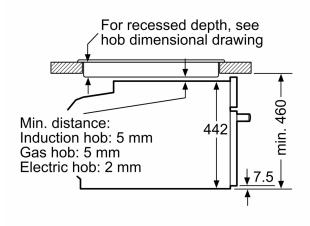
measurements in mm
