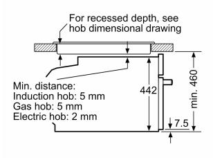
measurements in mm
