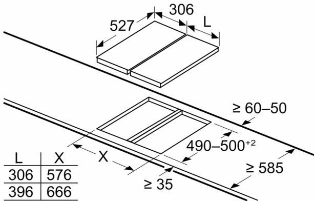
If two or more elements are installed right next to one another, one or several installation kits are required (2 elements 1 installation kit, 3 elements 2 installation kits, etc.)
