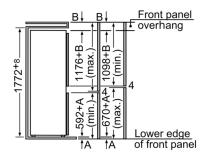
The specified unit door dimensions are valid for a door gap of 4 mm. If a different gap width is used (max. 14 mm), the dimensions must be adjusted.
