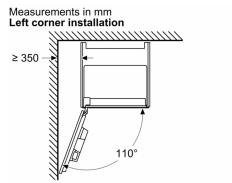
If using the 92° hinge limiter, the min. distance to the wall is only 100  $\,\mathrm{mm}$
