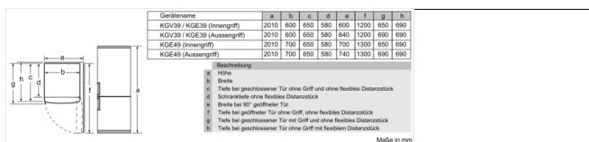
The diagram illustrates the front view of the refrigerator-freezer combination with various dimensions labeled: a (width), b (depth), c (depth of the left door), d (depth of the right door), e (width of the left door), f (width of the right door), and g (height). Below the diagram is a table of technical data:
