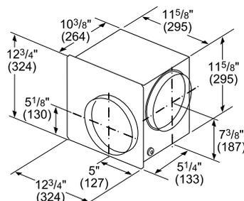
measurements in inches and (mm)
