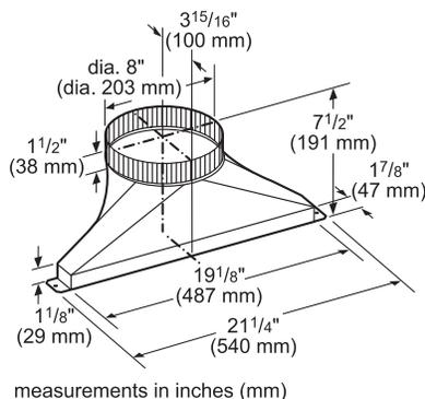
**NOTE:** Some applications may require deeper cabinets. Side and rear exhaust require at least 18" of clearance to fit the blower and / or ductwork. Refer to installation instructions.
