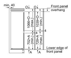
The specified cabinetry door dimensions apply for a door gap of 4 mm.
