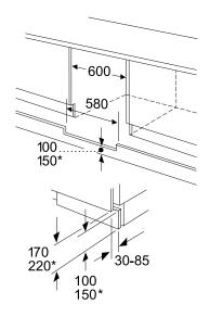
Space for electrical connection next to the appliance on the left or right-hand side. Ventilation space in the base.
