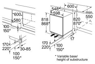
Space for electrical connection on the right side or on the left next to the appliance. Venting to and from the base.
