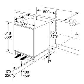
\* Variable base/substructure height
