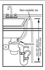
Note: Plumbing installations will vary - refer to local codes. Drain hose included is 75" (190 cm) and can be extended to a maximum of 151" (383 cm).
