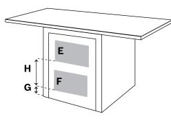
If the front of the appliance is covered, ventilation openings must be installed as shown and front/rear clearances adhered to according to closet installations.
