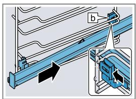
3. Press and hold **PUSH** ① and swing the pull-out rail inwards ② until the retainer ⓐ is attached in the lower rod.
