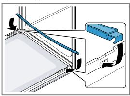
6. Note: When sliding the pane in, ensure that the glossy side of the pane is on the outside and the cutouts on the left and right are at the top. Slide the inner pane into the left- and right-hand retainers a.
