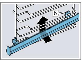
2. Guide the rail lengthways to the rear to the guide rods, and slide both retainers onto each lower rod. In doing so, use the rear retainer b to grip the vertical rod.
