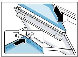
7. Push the inner pane upwards until it is in the left- and right-hand retainers a.
