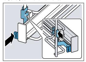
2. Press and hold **PUSH** ① and swing the rail outwards ② until the front retainer ② is detached.
