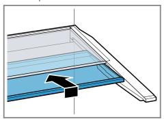
If more space is required, you can fold up the front and rear section of the variable shelf together.
