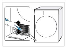
Ensure that you vacuum the fins from top to bottom so that they do not become deformed or damaged.
