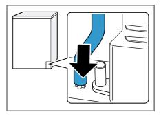
Push the water outlet hose as far as it will go into the connecting piece.
