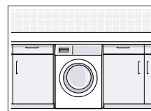
Only install the appliance underneath a continuous worktop that is securely connected to adjacent cabinets. Required niche width: 60 cm.
