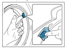
**4.** Clean the outside and the inside of the rubber gasket with a damp cloth and wipe dry.
