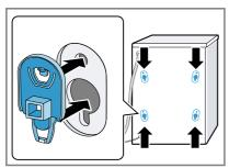
• If one cover cap is included in the scope of delivery, insert the cover cap in the bottom left opening for the transit bolt.
