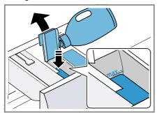
Do not exceed the marking for the maximum fill level when filling.
