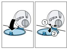
5. Slide a suitable receptacle under the opening for draining the detergent solution.
