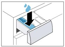
Add washing powder containing oxygen bleach to the manual dosing compartment.
