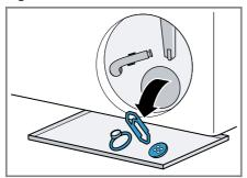
**3.** Ensure that both impellers can turn.
