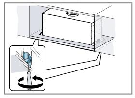
**3.** Screw in the front two screws and select a hole so that the surface of the appliance is flush with the fitted unit.
