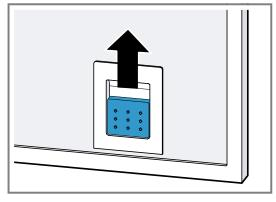
Remove the grease filters from the holders. To prevent grease from dripping, hold the grease filter horizontally.
