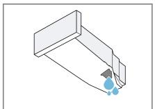
Check the condensation container filter regularly and clean the filter if it is dirty.  $\rightarrow$  *Page 38* Make sure that you insert the condensation container before operating the appliance.  $\rightarrow$  *Page 32*
