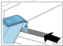
Observe the mark for filling the water tank next to the front opening. If ♠ does not go out on the display, align the appliance correctly. → "Aligning the appliance", Page 16
