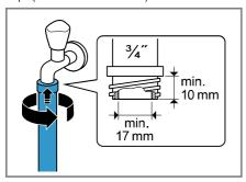
3. Open the water tap carefully and check that the connection points are tight.
