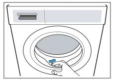
Leave the appliance door and detergent drawer open so that residual water can evaporate.
