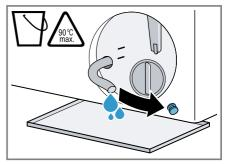
8. Firmly press on the sealing cap.
