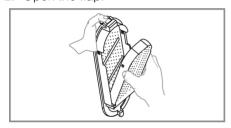
**3.** Clean the filter with running water and close the flap.
