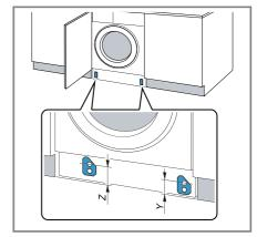
3. Screw the spacers in as per the dimensions.
