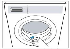
3. Clean the outside and the inside of the rubber gasket with a damp cloth and wipe dry.
