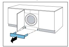
Slide a suitable receptacle under the opening for draining the detergent solution.
