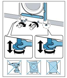
**9.** Tighten the lock nuts on the front appliance feet hand-tight against
