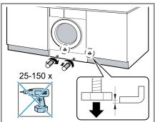
**8.** Align the appliance using a spirit level.
