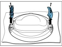
**3.** Screw the door hinge and the door hook onto the opposite sides.
