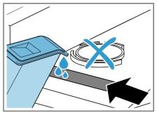
Check the water tank filter regularly and clean the filter if it is dirty. → "Cleaning the water tank filter", Page 44
