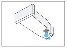
Check the condensation container filter  $\rightarrow$  Page 45 regularly and clean the filter if it is dirty. Make sure that you insert the condensation container before operating the appliance.
