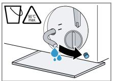
8. Firmly press on the sealing cap.
