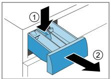
3. Pull out the insert upwards.
