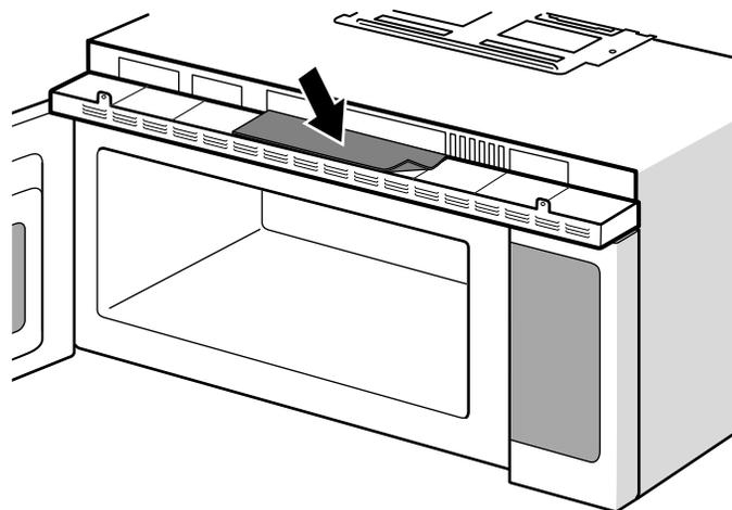
5. Carefully push the vent grill back into place and replace the screws removed in Step 2.
