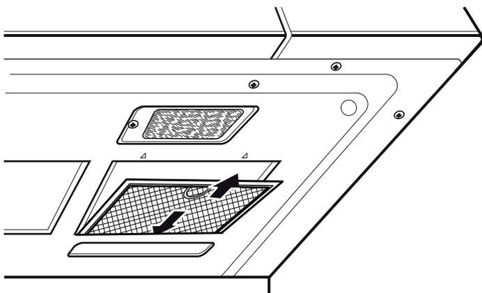
2. Soak the ventilation filters in hot water using a mild detergent. Rinse well and shake to dry. Do not use ammonia or wash in a dishwasher. The aluminum on the filter will corrode and darken.
