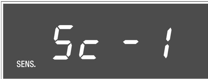
When sensing is complete, two short beeps will sound and the calculated cook time will start to count down.
