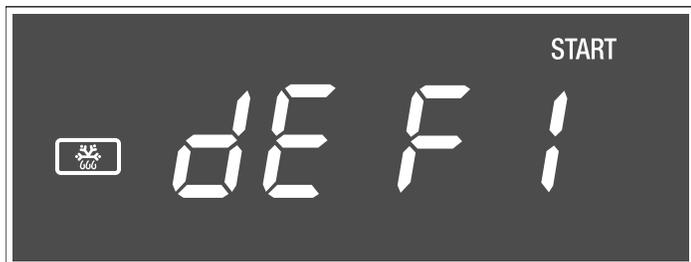
2. Touch **Auto Defrost** repeatedly until the desired program number is shown in the display. Check the menu label at the bottom of the appliance cavity or see program table below.
