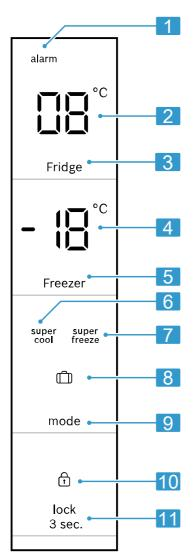
alarm lights up when the alarm is switched on.
