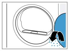
3. Remove the two-part fluff filter.
