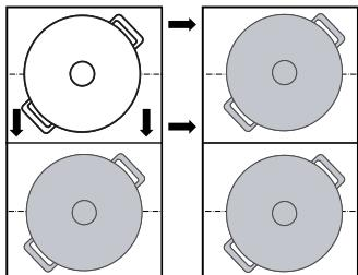
The cookware is detected and the previously selected power level and  $\text{t}$  flash alternately on the display for the new cooking zone.
