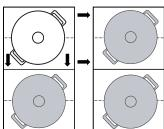
The cookware is detected and the previously selected power level and £ flash alternately on the display for the new cooking zone.
