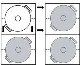
The cookware is detected and the previously selected power level and £ flash alternately on the display for the new cooking zone.
