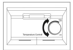
**Note:** At a room temperature above 32 °C, slightly reduce the temperature setting in the appliance. At a room temperature below 16 °C, slightly increase the temperature setting in the appliance.
