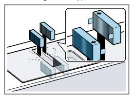
6. Insert the grease filter.
