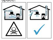
Always ensure adequate fresh air in the room if the appliance is being operated in exhaust air mode at the same time as a room-air-dependent heat-producing appliance is being operated.
