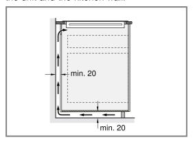
Ensure that an opening at the top of the rear of the unit is unobstructed.
