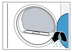
3. Remove the two-part fluff filter.
