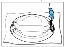
When you do this, ensure that the door seal is not trapped or damaged.
