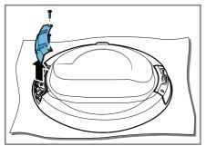
2. Unscrew the door hinge and the door hook.
