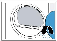
3. Remove the two-part fluff filter.
