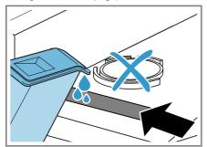
Check the water tank filter regularly and clean the filter if it is dirty. → "Cleaning the water tank filter", Page 51
