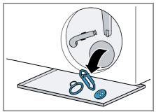
**3.** Ensure that both impellers can turn.
